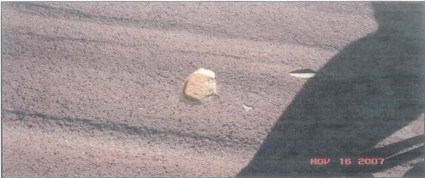
79. This photograph shows the separated layer of the foam. The foam is wet.
